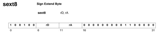
This instruction sign-extends a byte (8 bits) into a word (32 bits). Bit 24 in rA will be copied into bits 0-23 of rD. Bits 24-31 in rA will be copied into bits 24-31 of rD.
